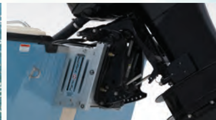
Hydraulic jack plate (shown on 21 LTS)
