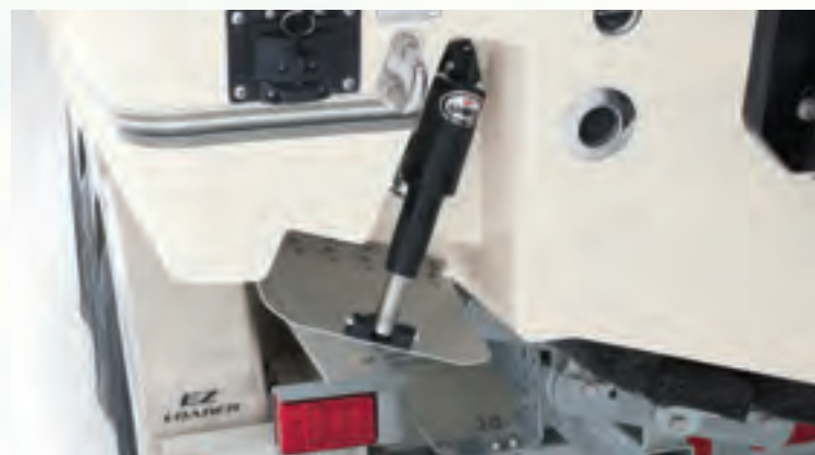
Boat-leveling trim tabs (shown on 284 CC)
